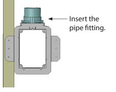
The pipe fitting is designed to slide in the frame to adjust for variations in wall board thickness.
