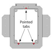
Insert the valve assembly into the rough-in frame.
