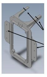
Push the bottom two pointed tabs into the sheetrock. The top pointed tab can be bent down as you pull the top of the frame into the hole. The tabs will help hold the frame in place while you install the valve. You may need to push a couple of small finish nails, horizontally into the sheetrock, through the holes located on the side of the frame.
